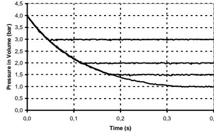
Fig. 15: Pressure Control (Decreasing Pressure)
