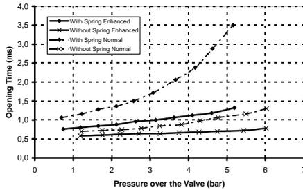
Fig. 8: Opening times of valves
