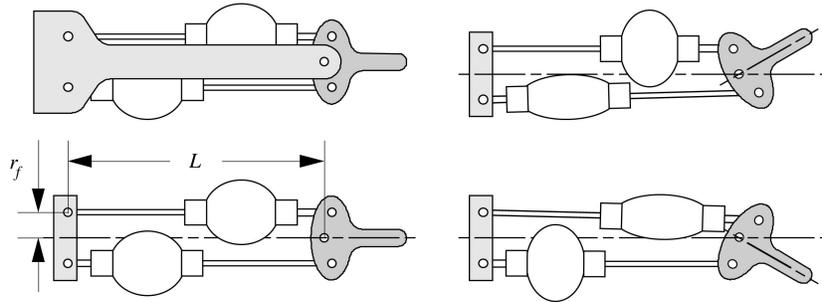
Fig. 17: Rotative joint actuated by 2 antagonistic PPAMs
