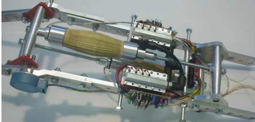
Fig. 23: Modular part, configured as knee joint
