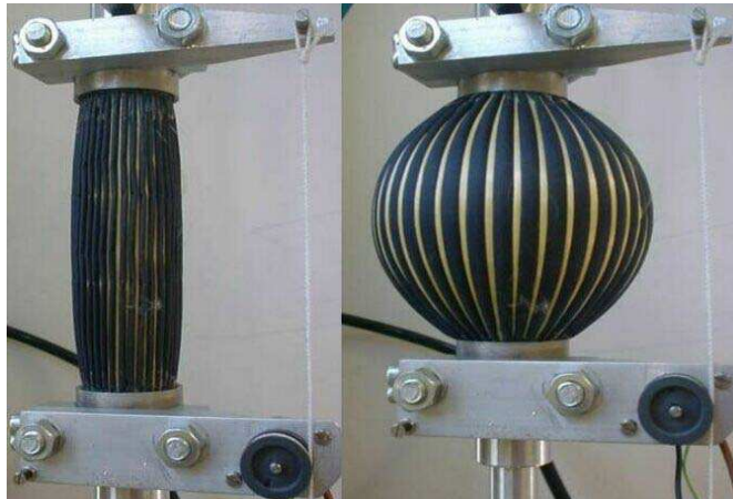
Fig. 1. photograph of deflated and inflated state of the PPAM
