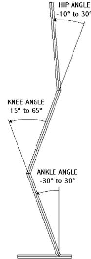
**Fig. 9 Range of motion for the joints**
