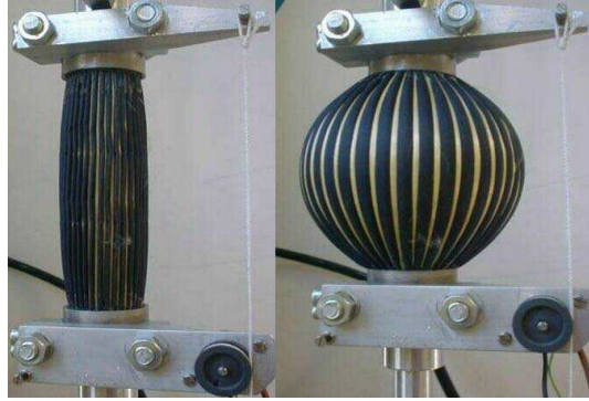
Fig. 2. Photograph of deflated and inflated state of the PPAM
