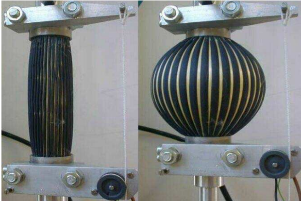
Fig. 1. Deflated and inflated state of the PPAM
